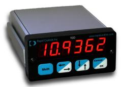
The TDD2 displays position information derived from a magnetostrictive transducer with Synchronous Serial Interface (SSI), Start/Stop, Pulse Width Modulated (PWM), or CANbus output. Setup of units, offsets, and other items can be accomplished via the front-panel keypad menu or a RS-232/485 interface.
