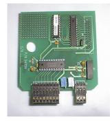
OPTIONAL LIMIT SWITCH and ANALOG BOARD INDUCTIVE KICK BACK Protection. Failure to provide adequate kickback protection for relays, motors etc. can cause the TDD to lock up or damage the output transistors.
